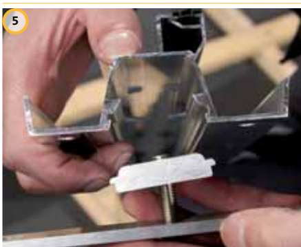
5 Snap rotation anchors into side member and mark fixation point
